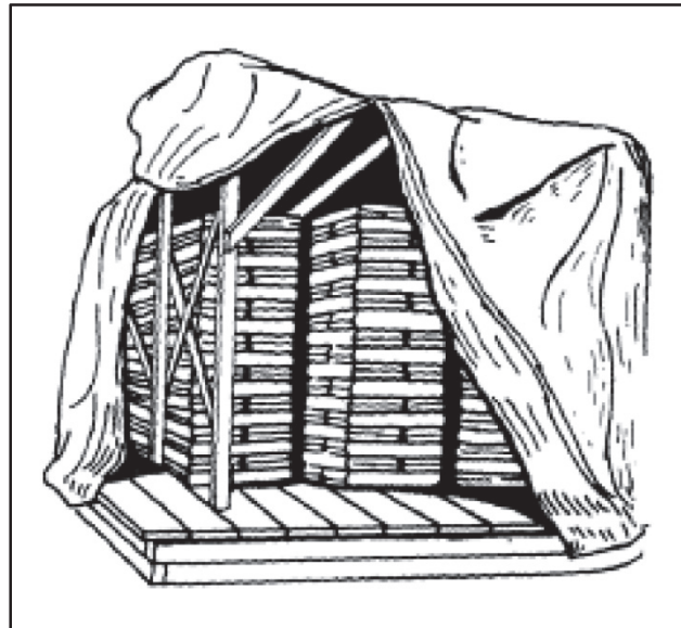
Figure 8-1. Cement stored under tarpaulins
